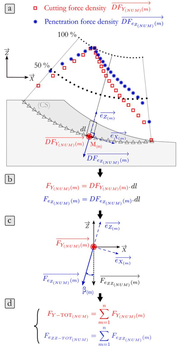
Fig. 8. Macroscopic numerical forces building given a cut section CS and forces distribution extracted from 2D ALE cutting models.
