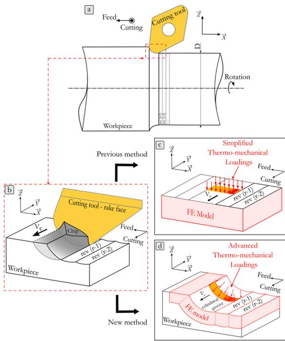
**Fig. 1.** Principle of the residual stress modelling based on a two-scale approach. a) longitudinal turning operation, b) zoom on the chip formation zone, c) turning operation modelling based on equivalent thermo-mechanical loadings (previous method) (Mondelin et al. (2012)), d) turning operation modelling based on new advanced equivalent thermo-mechanical loadings (new method).
