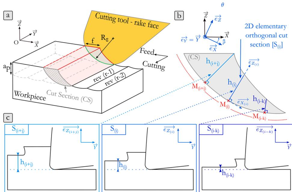
Fig. 4. Geometrical approach to discretise the cutting edge in several 2D elementary orthogonal cut sections. a) material removal description, b) theoretical undeformed cut section CS and 2D sections  $S_{(i)}$  parametrisation along the cutting edge, c) example of 2D sections  $S_{(i)}$  with the corresponding uncut chip thickness  $h_{(i)}$ .
