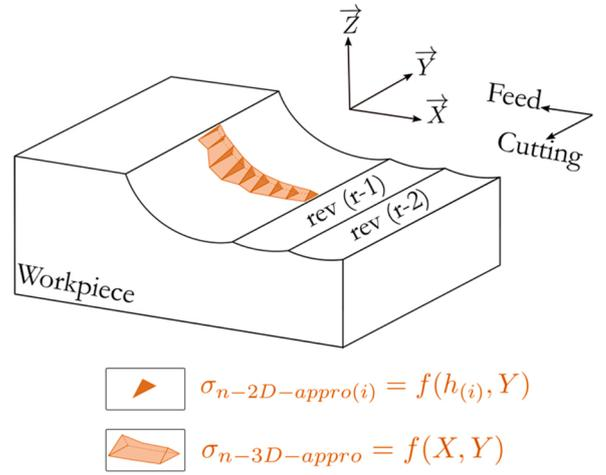
Fig. 7. 3D thermo-mechanical shapes building - example of the normal pressure (see Fig. 6).
