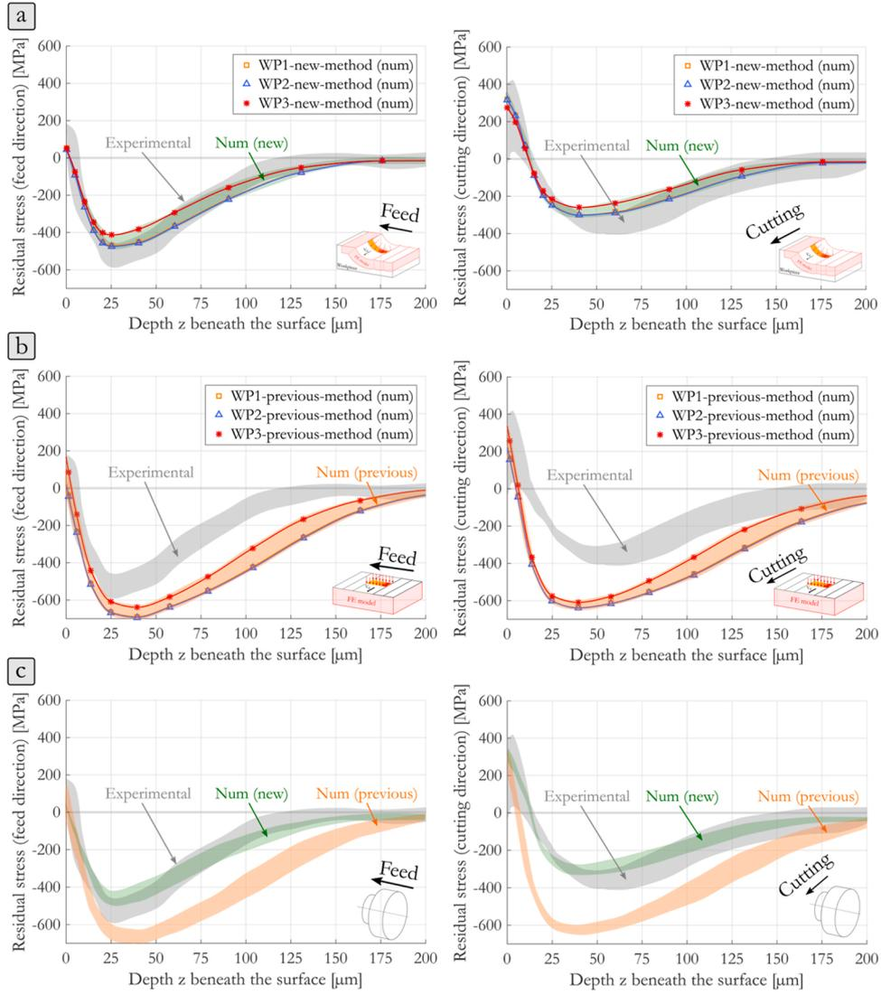
**Fig. 15.** Residual stress comparison for numerical model validation, experimental results are displayed through the grey cloud and compared for the three workpieces with a) the new numerical predictions, b) the previous numerical predictions, c) overview of the accuracy of both numerical methods predictions compared to the experimental results.
