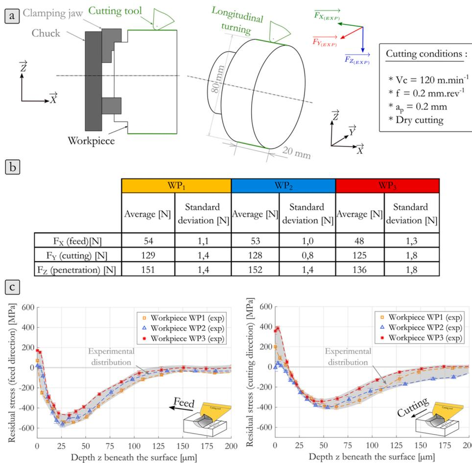
Fig. 13. Model validation experimental case description. a) case-study with cutting conditions, b) macroscopic experimental turning forces for three turning tests, c) residual stresses profiles beneath the surface in two directions.
