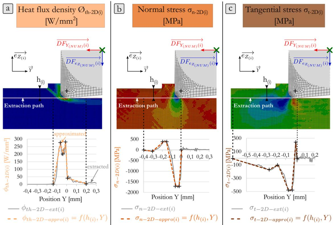
Fig. 6. 2D equivalent loadings and turning forces densities extractions from 2D ALE cutting models. Given an uncut chip thickness  $h_{(i)}$  at point  $M_{(i)}$  located in the cutting edge and for each considered equivalent loading, linear approximation of the complex extracted shapes, a) heat flux density  $\phi_{th-2D-appro(i)}$ , b) normal pressure  $\sigma_{n-2D-appro(i)}$ , c) tangential pressure  $\sigma_{t-2D-appro(i)}$ .
