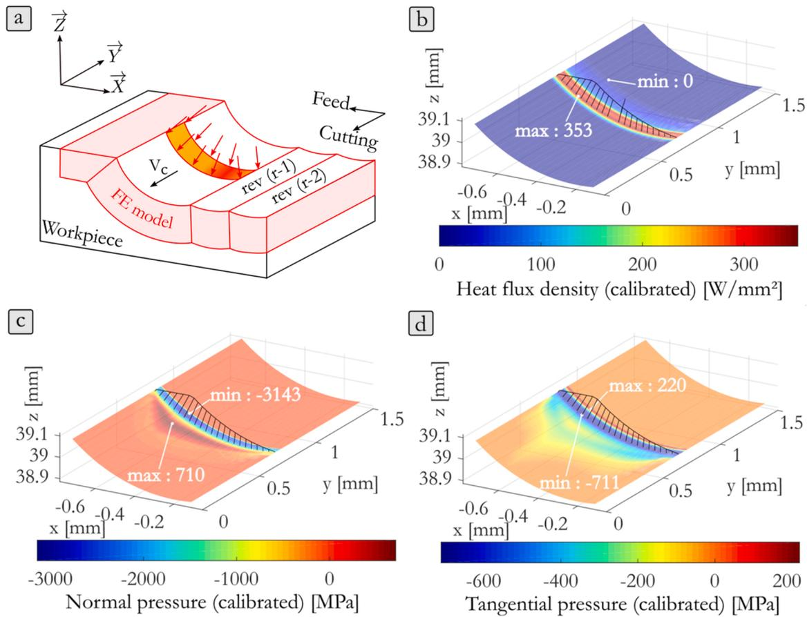
Fig. 10. Final 3D equivalent thermo-mechanical loadings description with physical shapes and corrected intensities. a) finite element model, b) heat flux density, c) normal pressure, d) tangential pressure.
