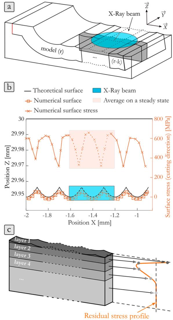
**Fig. 14.** Numerical residual stress profiles building methodology, a) model overlapping of successive revolutions, b) surface residual stress average on a stabilised zone, c) in-depth average layer by layer for residual stress profile building.
