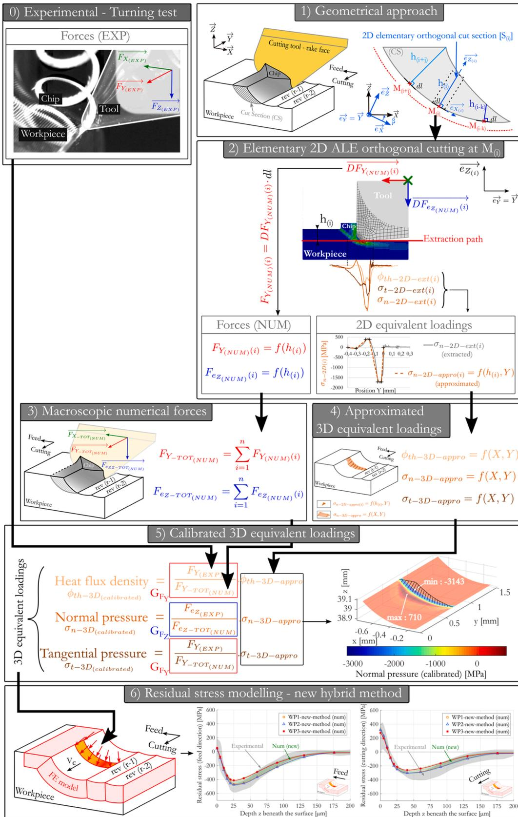
Fig. 3. Flowchart of the new 3D hybrid methodology through steps number zero to six.
